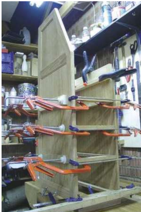
▲ Pic.9 The left-hand outer and inner frames assembled with as many cramps as you own!
